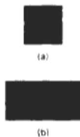
Figure 5-6 Turning a square (a) into a rectangle (b) with scaling factors s_x = 2 and s_y = 1 .
